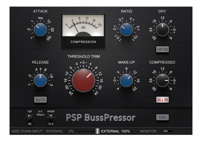
**Compression Meter:** This meter displays the compressor's average gain reduction level.
