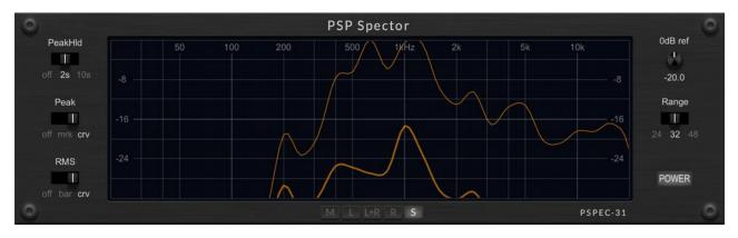
**NOTE**: Although the curve mode may resembles a Fast Fourier Transform (FFT) display, it is still a 1/3-octave measurement, interpolated for a smooth overview curve on the display.
